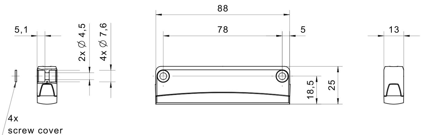
With safety sensor 165 ESK 00. 3. the actuator is programmed on the sensor. After this process has been completed, the sensor detects only the programmed actuator.
