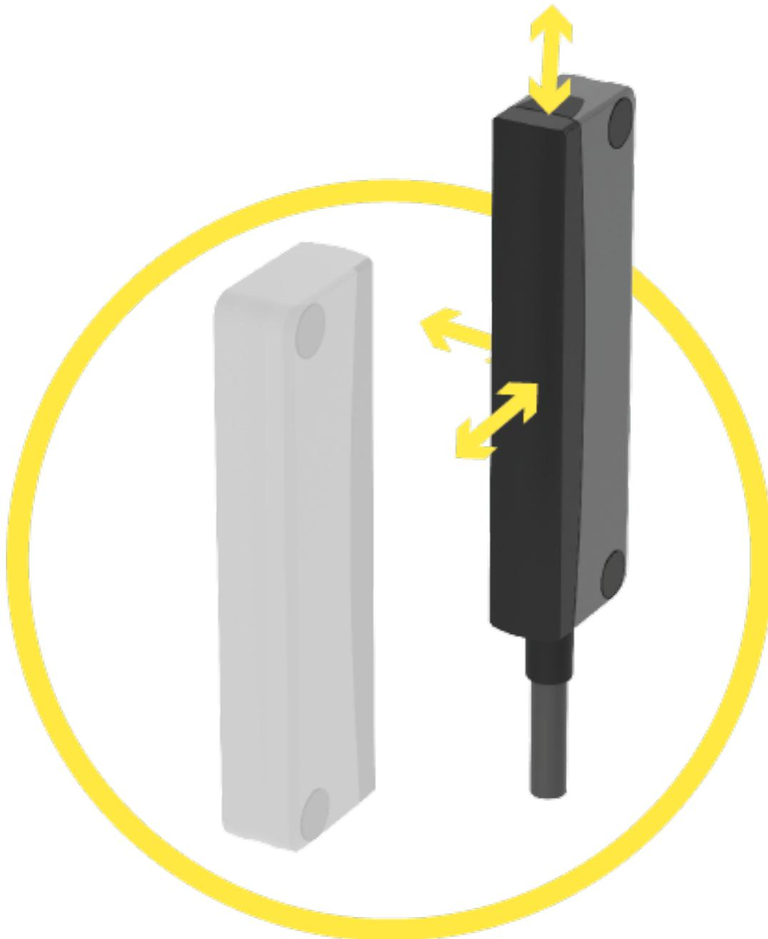
Suitable for front, side and 90° actuation. Operating distance (Sao) from 5 to 14 mm. Assured switch-off distance (Sar) from 8 to 18 mm.
